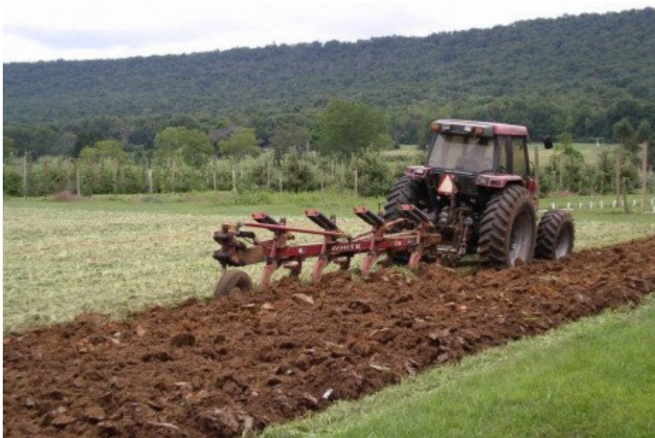
Moldboard plowing, shown here, is a type of primary tillage. Photo courtesy of Penn State Extension
